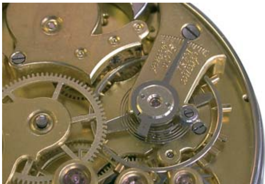
3. Breguet overcoil balance spring with index regulator.
