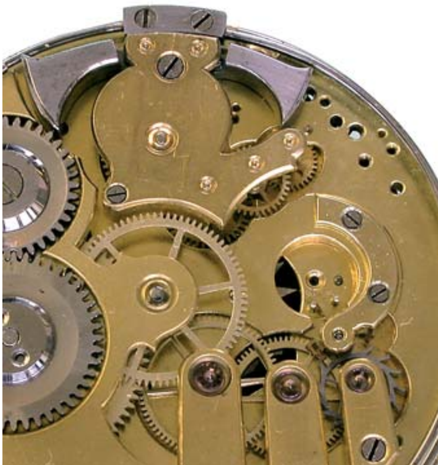
5. Modern in line lever and escape wheel. Also the repeat barrel, governor train, hammers and gongs. The balance has been removed.
