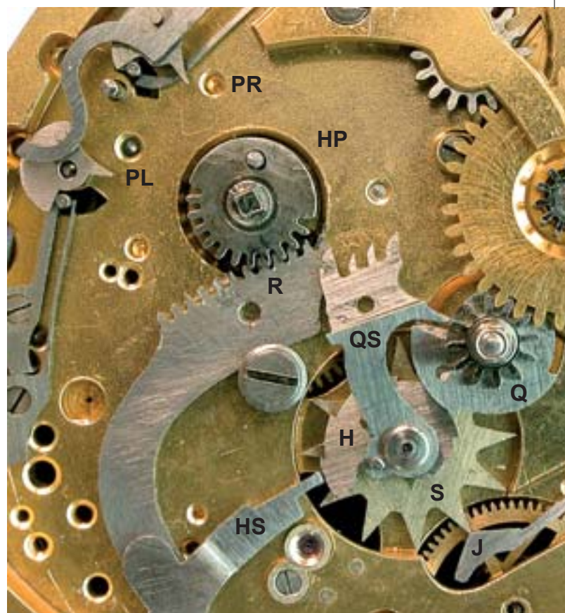
7. The hour and quarter snails and stops, just before the hour, the surprise piece not showing.
