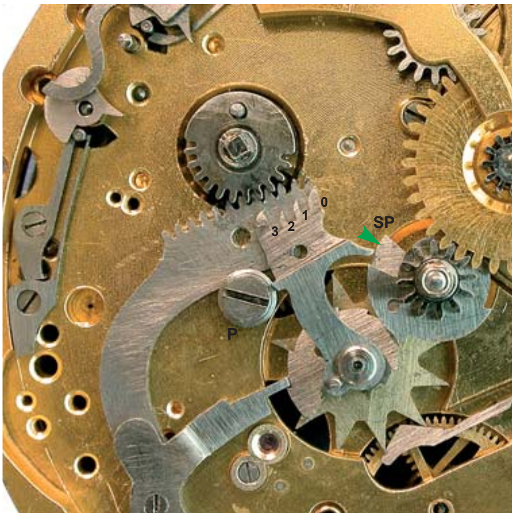
8. The snails just after the hour, when the surprise piece has shot out, arrow.
