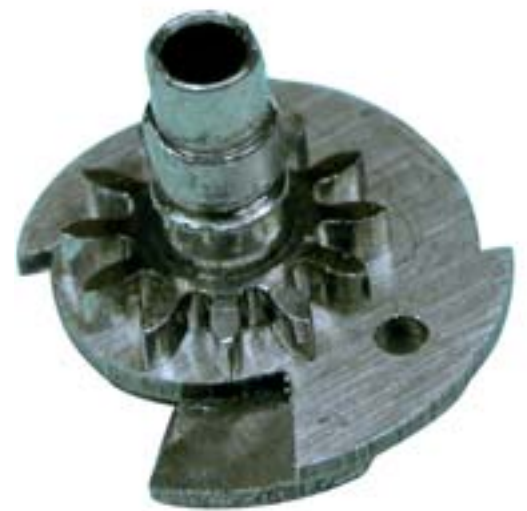
9. Close up of the cannon pinion and quarter snail, with the surprise piece extended.
