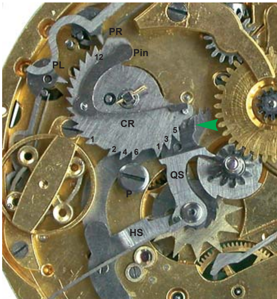
10. The strike rack and pawls, also the hour and quarter stops.
