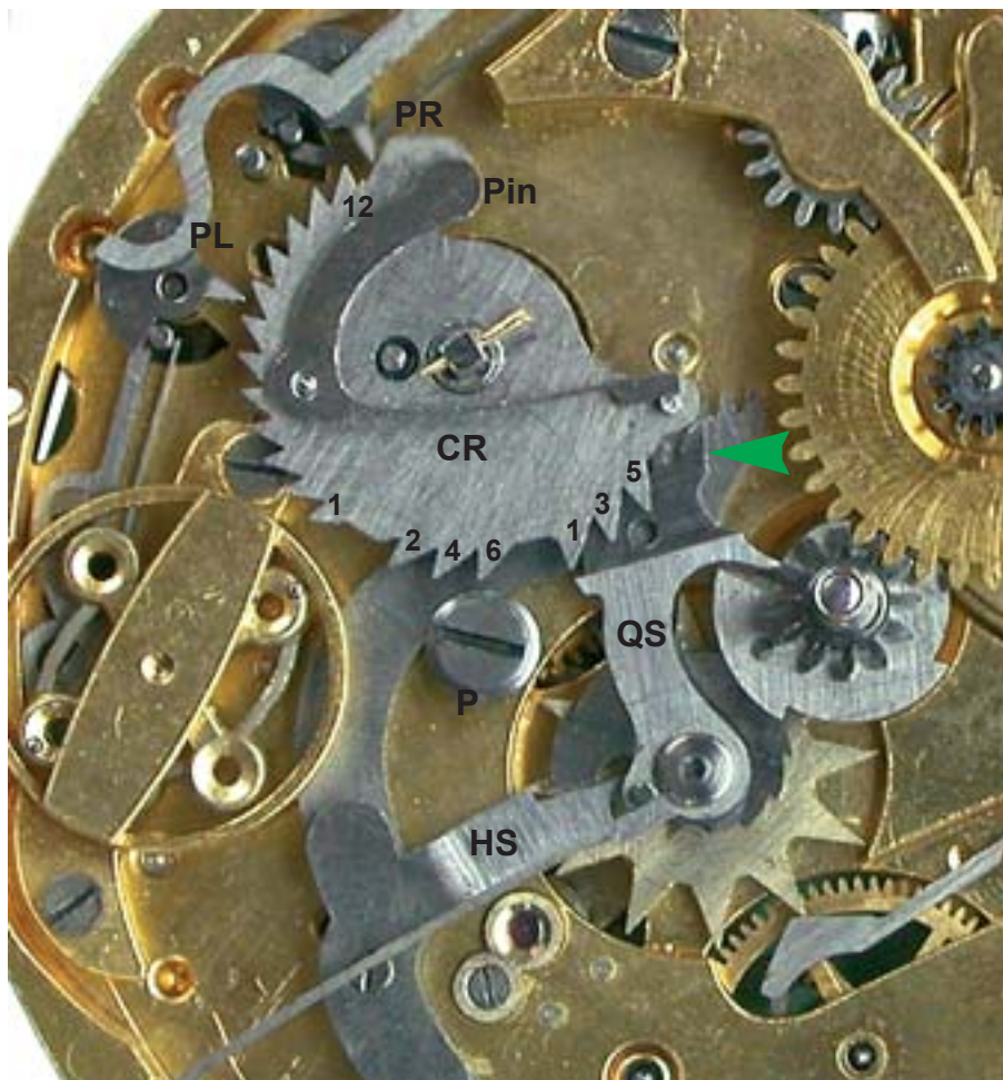
10. The strike rack and pawls, also the hour and quarter stops.
